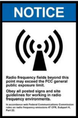
3 RF GUIDELINES SIGN - 12" X 8" - PLACED ON FENCE
