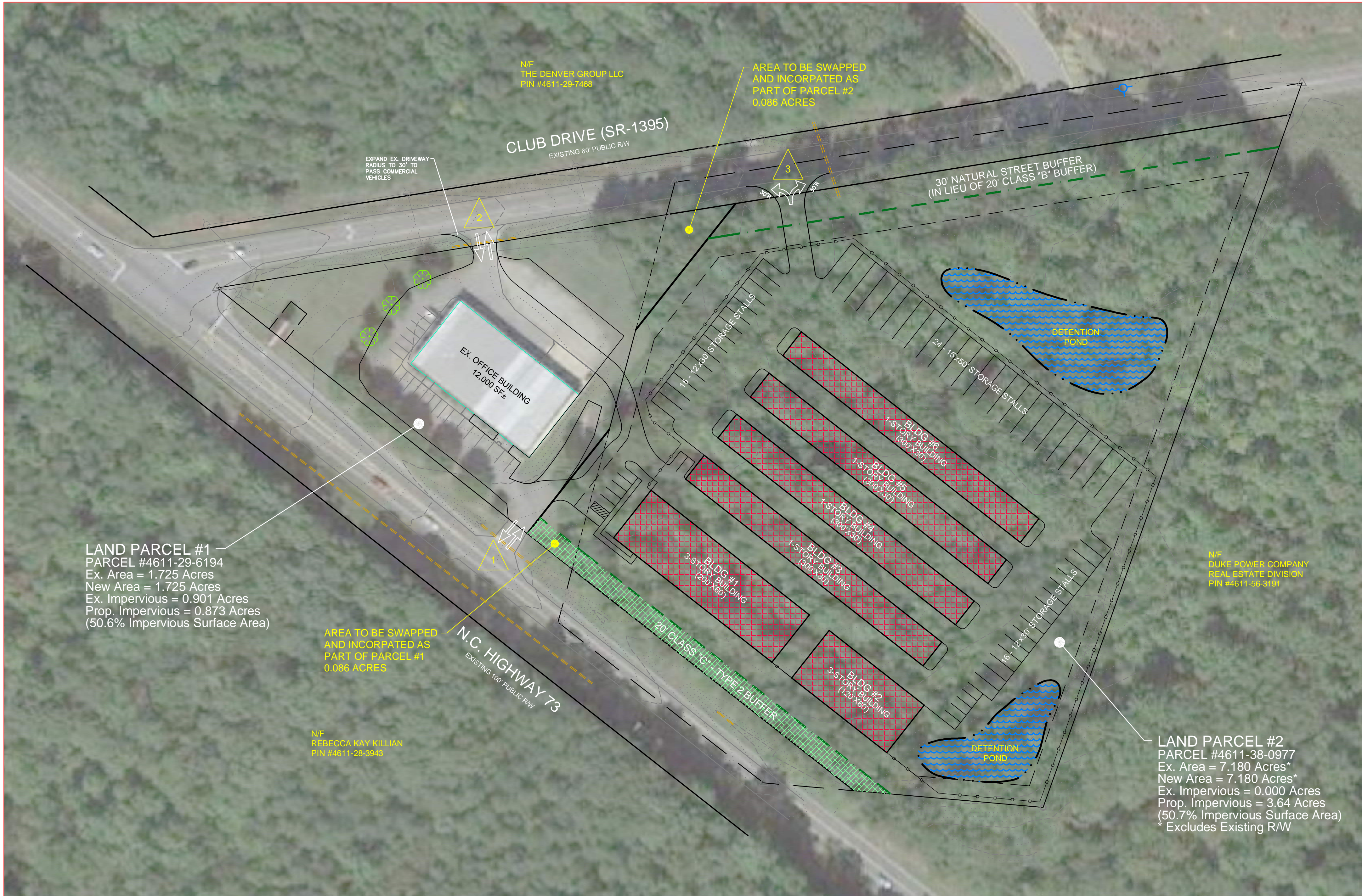
TYPICAL BUFFER: HIGHWAY 73 20' CLASS "C" - TYPE 2 3'-4' EARTHEN BERM 1 LARGE CANOPY TREE PER 100LF 1 EVERGREEN TREE PER 100LF 1 UNDERSTORY TREE PER 100LF 12 SHRUBS PER 100LF
